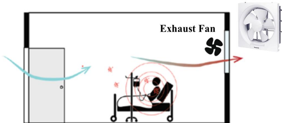
Figure 4: Exhaust fan placed on the wall at the patient's head end to draw the air from clean to less clean.
