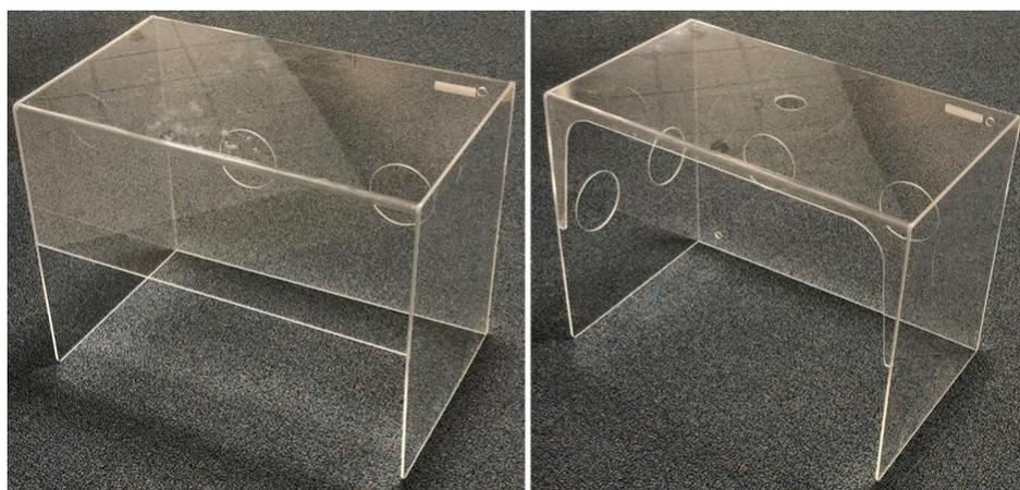
**Figure 4:** The early-generation aerosol box (left) and the latest-generation aerosol box (right) which were studied.<sup>9</sup>
