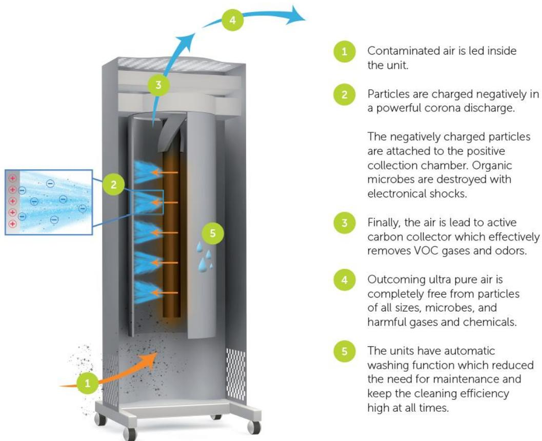
**Figure 1: Basic working mechanism in Genano portable air decontamination units<sup>2</sup>**
